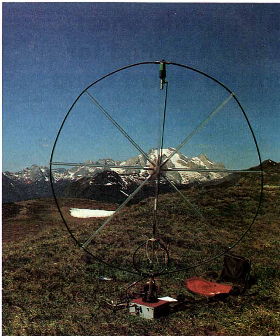
The short loop antenna in operation from the Italian Eastern Dolomites at 2250m above sea level. It is light in weight, and easily dismantled for transportation.
